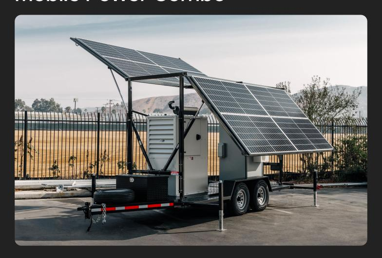
Whether you are operating a Private LTE, WiFi, Commerical Cellular or just need power, there is no better solution to getting on-air faster than the HyBridge Gen2. The trailer features a powerful hybrid energy system combining solar, generator and batteries enabling silent, fossil fuel-free operation during low energy phases boasting a fuel cost
